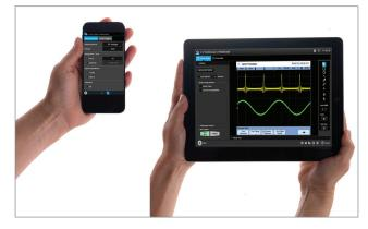
**BenchVue Mobile** is a mobile app that you can install on an Android or Apple iOS device to control BenchVue bench applications running on your Windows computer. BenchVue Mobile connects to your computer as a client, and requires that your mobile device and computer be connected to the same local network or intranet (behind the same corporate firewall). This network connection can be made via a WiFi connection inside your work location or externally through a VPN connection.
