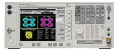
2001 | PSA spectrum analyzer
