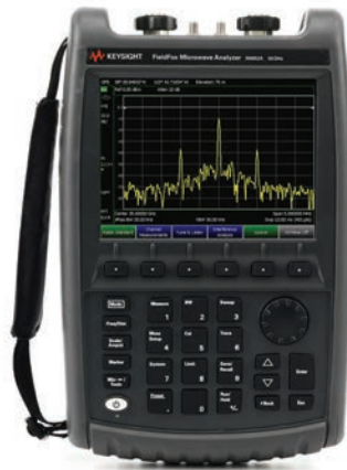
2015 | FieldFox 50 GHz handheld microwave analyzer
