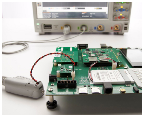
N2820A high-sensitivity 2-channel current probe
