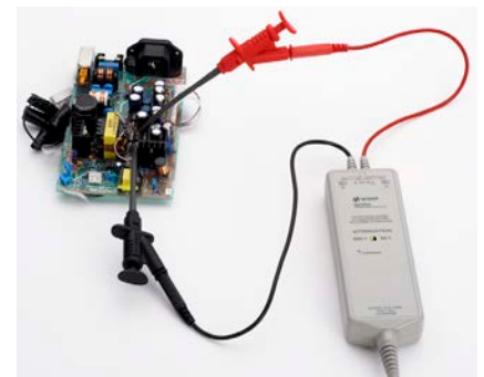
N2790A measuring a power supply signal
