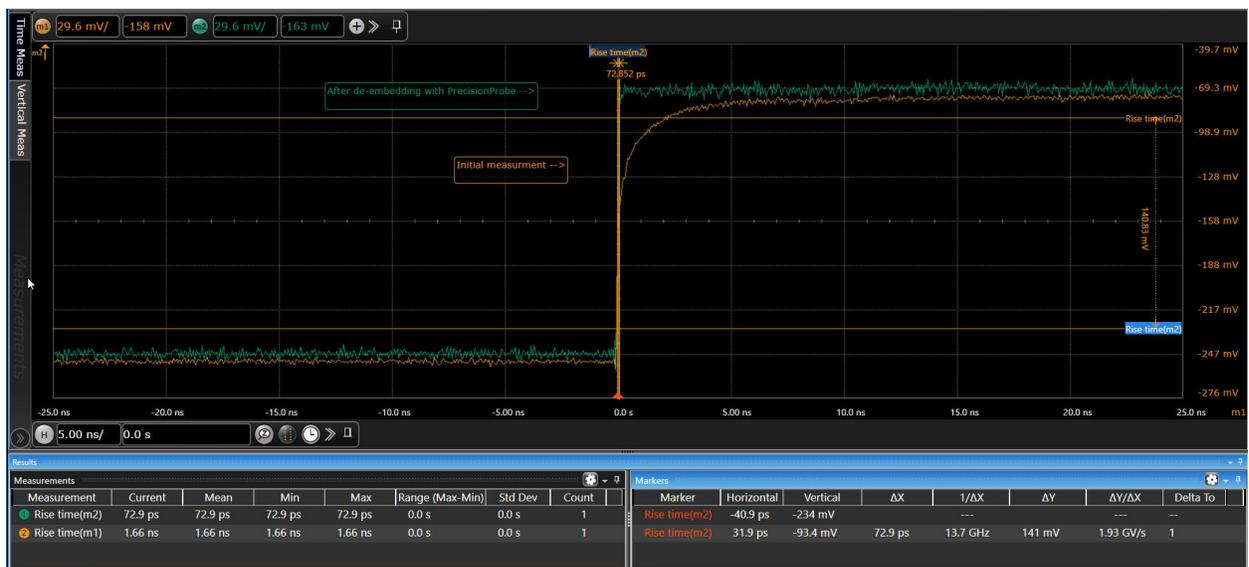
This package includes PrecisionProbe and InfiniiSim Basic, two tools designed to de-embed the effect of cables and fixtures from measurements. PrecisionProbe allows you to characterize the response of a probe, cable or fixture; InfiniiSim lets you model them out of a measurement.
