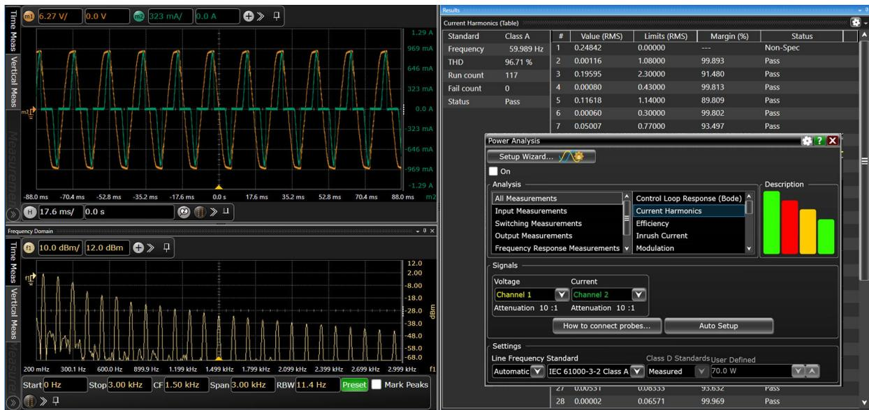
This application enables a broad range of automated power supply characterization measurements from input analysis, switching device characterization, and output analysis. It also includes critical frequency response measurements such as power supply rejection ratio (PSRR) and control loop response.
