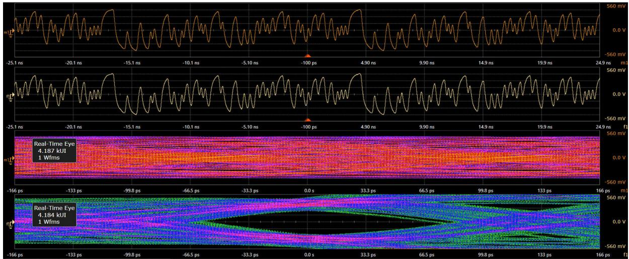
This package is intended for anyone working in high speed digital applications where eyes are closed. Equalization, InfiniiSim, and Crosstalk/Power Integrity packages enable deep analysis as to why an eye is closed, what it will take to open it, and simulating the results.
