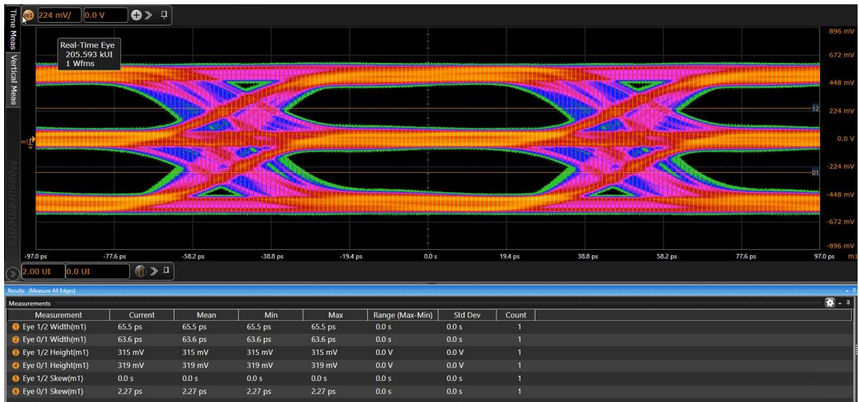
This package quickly sets up clock recovery and measurements for a PAM encoded signal. The software is also able to accurately set the individual threshold levels of your PAM signal and render each individual eye. It also includes BER/SER measurements and statistics.
