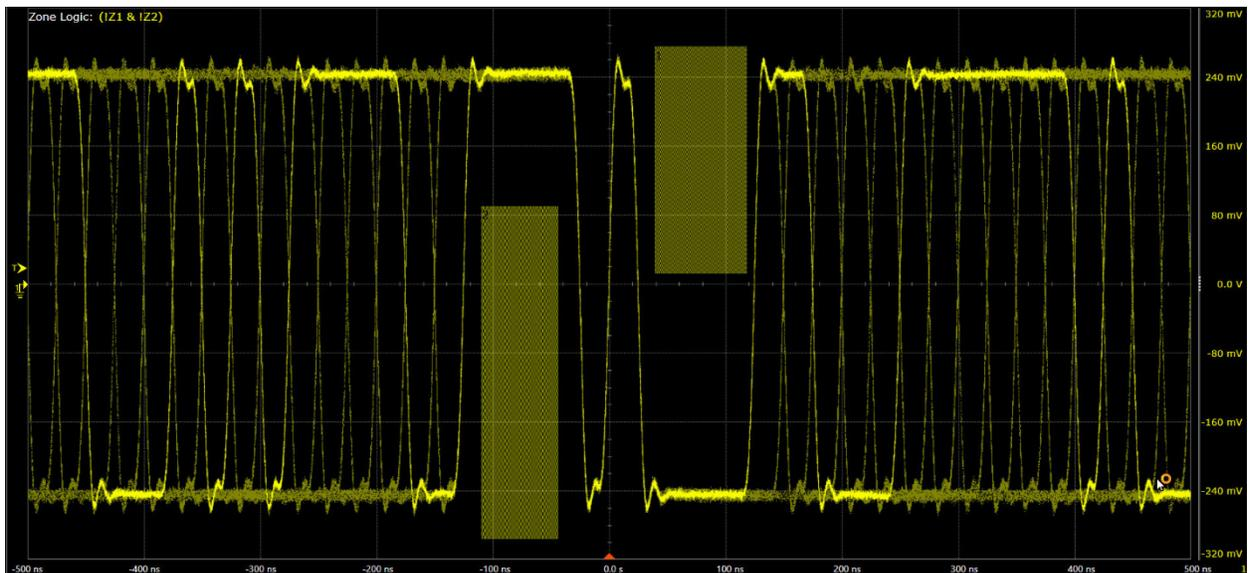
This package allows you to create a three-stage trigger to identify signal integrity issues that hardware triggering is unable to find in your electronic designs. This innovative software scans through thousands of acquired waveforms per second to help you isolate signal anomalies, saving you precious troubleshooting time. Trigger by drawing on-screen regions for a signal to hit or miss, or based on measured parameters.
