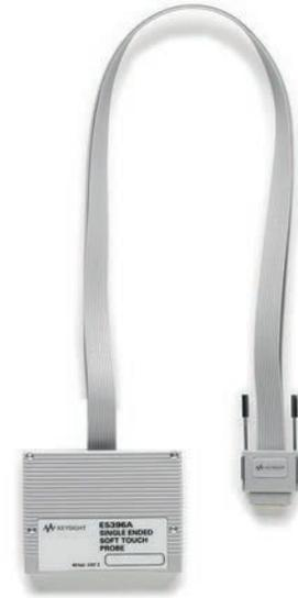
E5396A 16-channel soft touch connectorless probe
