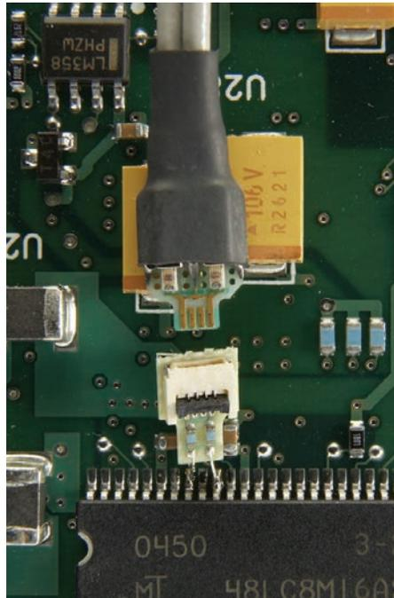
InfiniiMax ZIF tip soldered on board
