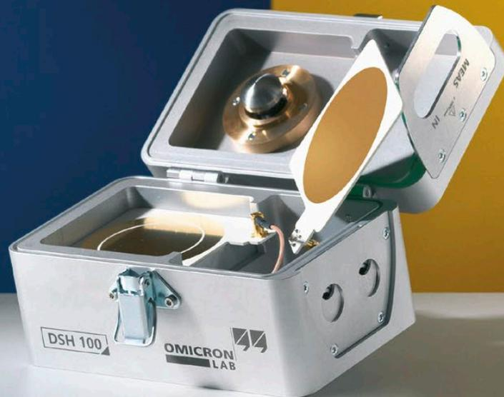
The **Dielectric Sample Holder DSH 100** is designed to analyze solid dielectric materials.
