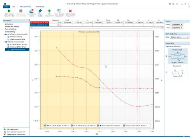
An **automatic compensation of parasitic capacitances (e.g. stray capacitances)** based on an air or reference material measurement ensure an easy handling and accurate measurement results.
