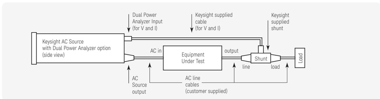
Test configuration of efficiency measurement using a Keysight AC source with the O20 Dual Power Analyzer Option.
