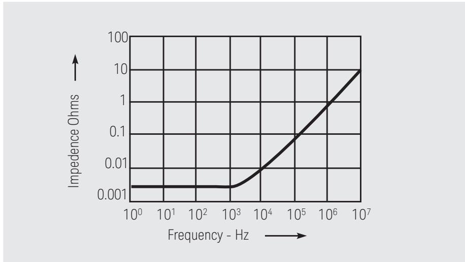
Typical output impedance of a constant voltage power supply
