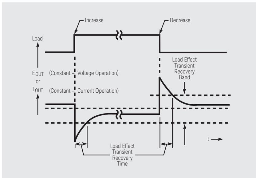
Load effect transient recovery waveforms
