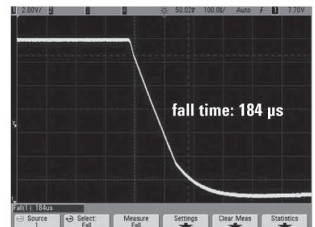
Figure 5. Pulse fall time of < 200  $\mu$ s
