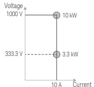
Figure 2. Rectangular output characteristic
