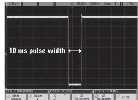
Figure 4. Voltage interrupt pulse
