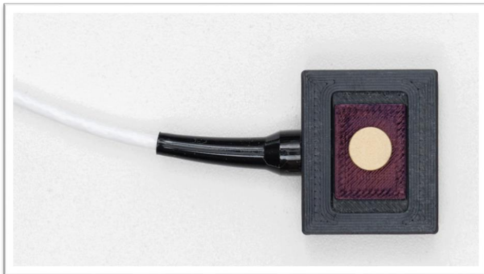
Figure 2: SEN-3D-CAM-CBL head with a sample
